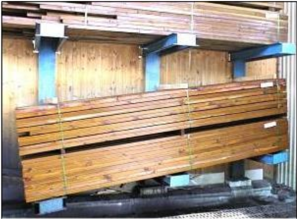
Pic. 8 Treated wood secured by PET
