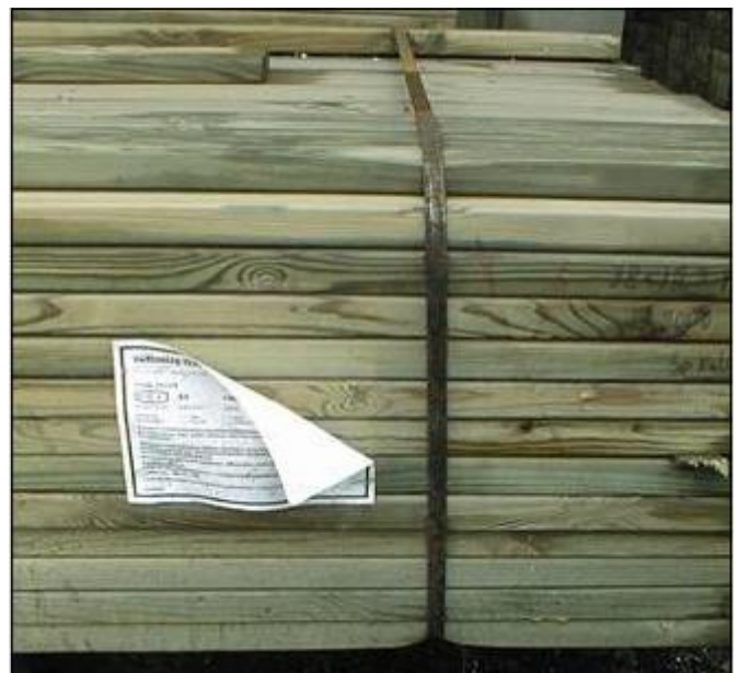
Pic. 2 Rust contamination and damaged
