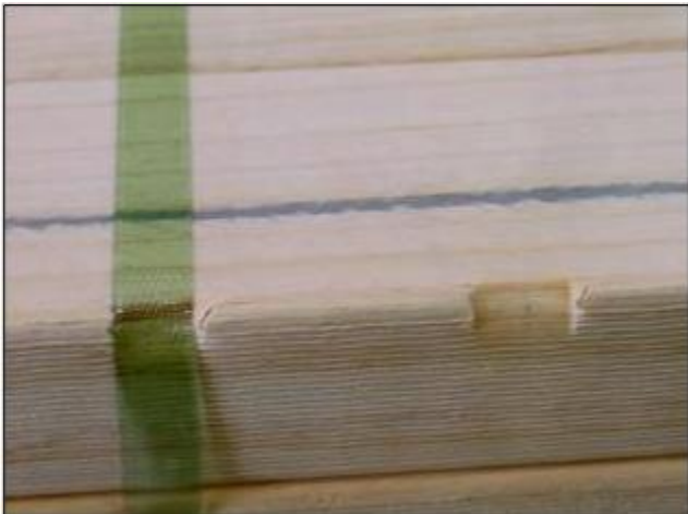
Pic. 7 Corner damage PET / Steel Strap comp
