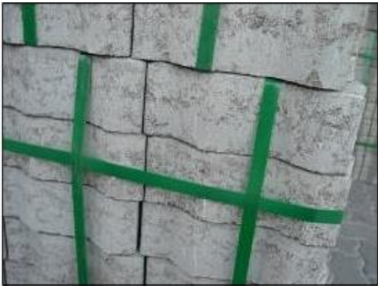
Sharp edges do not cut the strap
