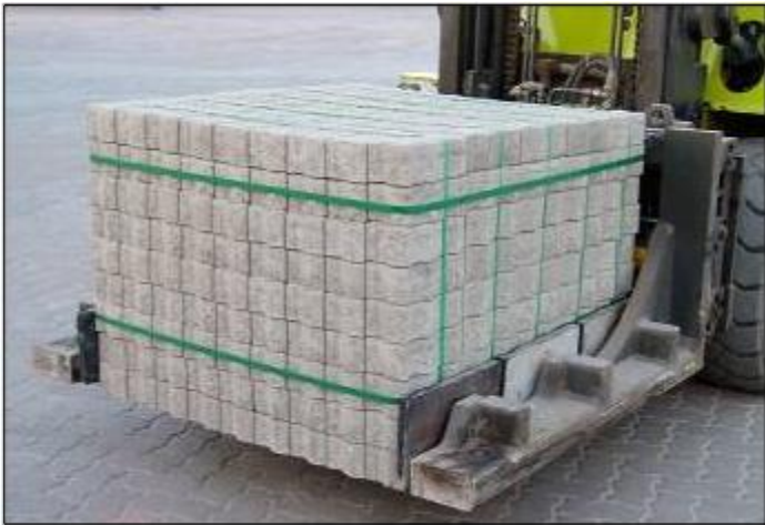
Lifting test: no sacking through
