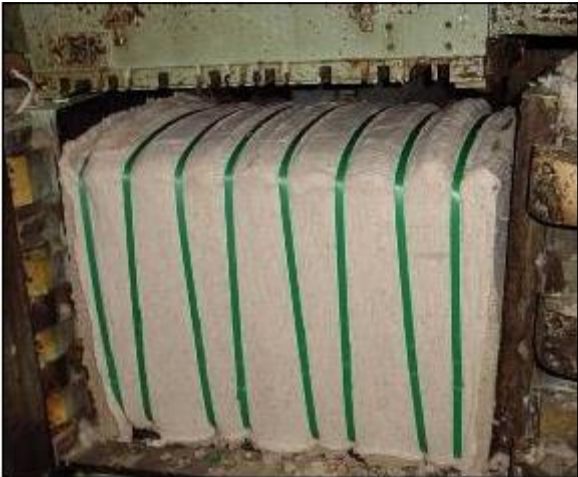
Press opens, straps are tensioned
