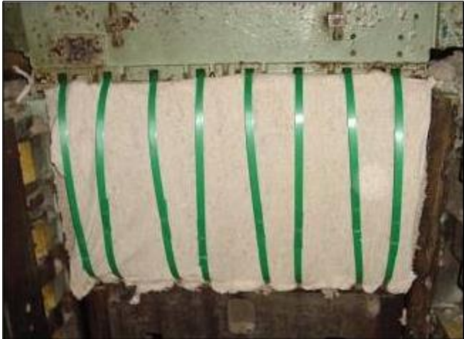
6 straps sealed loosely in press
