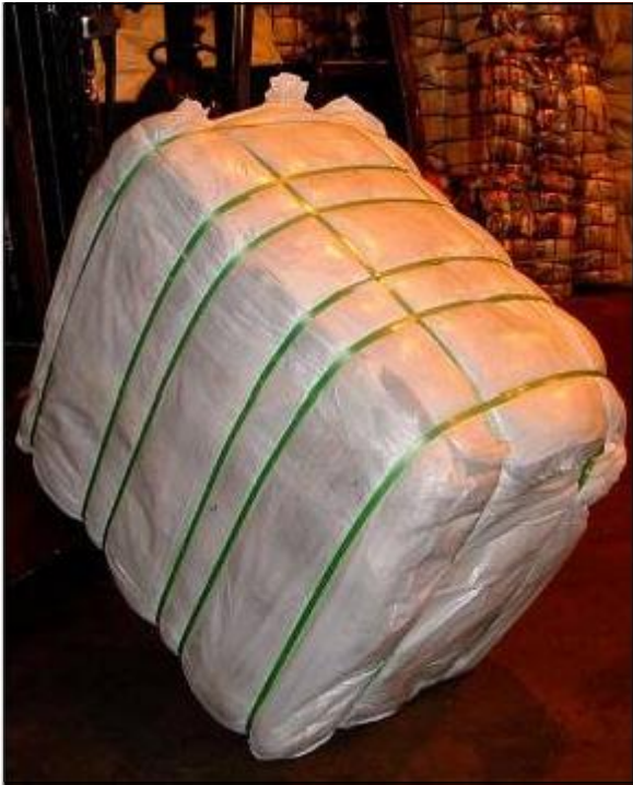
Large and small Textile Bales secures with PET strapping
