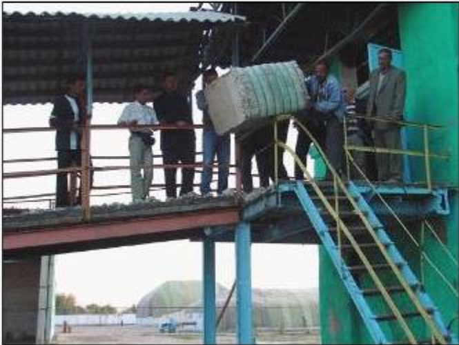
Fall test from a height of 4 m
