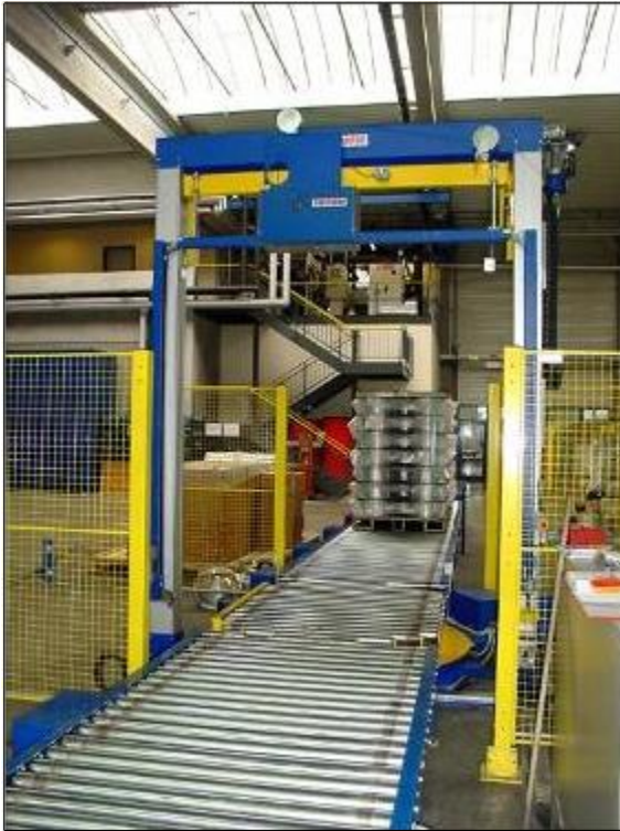
Conveyor and turn table
